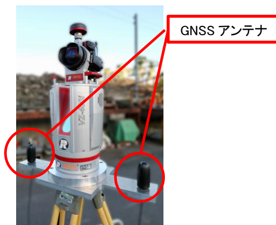
図2-6 GNSS-TLS
